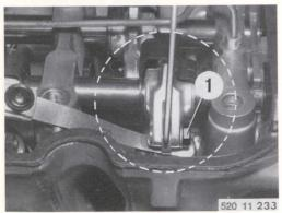
The order of adjustment is the same as the firing order: 1-5-3-6-2-4, and is carried out at top dead center (TDC) on the compression stroke. Adjust valve clearance between the valve and the eccentric after slackening off nut (1). Tighten nut (1) with special ring spanner 11 1 150 used in conjunction with torque wrench 00 2 050.
