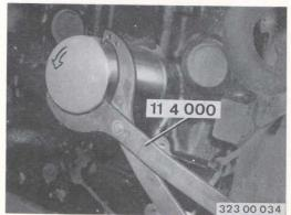
For version with air conditioning: Unscrew adaptor with a 32 mm ( $1^{1}/_{4}$  in) wrench and separate filter from adaptor.
