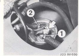
Unscrew fuel suction device by applying two crossed screwdrivers and turning counter-clockwise.
