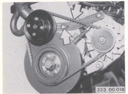
The V-belts when tightened correctly must yield under thumb pressure by 5 to 10 mm (0.2 to 0.4 in) at a point midway between two pulleys. Tighten V-belt for alternator and, if applicable, vane pump. Loosen alternator and, if applicable, vane pump, swing outward and retighten the bolts.
