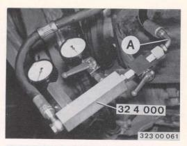
Connect pressure line (B) from pressure tester to vane pump. Close cut-off valve (1). Open cut-off valve (2) and bleed hydraulic system while engine is running at idle speed – 32 13 006. Engine must be at operating temperature for this. After bleeding has been completed, close cut-off valve (2) for max. 10 seconds and read the pressure. The pressure 1) given on the vane pump's data plate must not drop by more than 10%.
