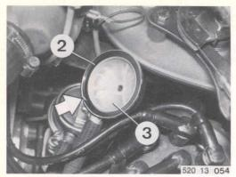
Remove cover with sealing ring (2) and strainer (3).
