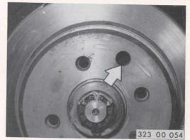
Insert a screwdriver and engage with the teeth on the adjusting nut.
