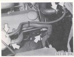
Take up slack at all hose clips on radiator an coolant expansion tank.
