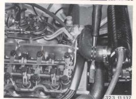
Adjust valves in same sequence as firing order (1-5-3-6-2-4), at compression to dead center (TDC).
