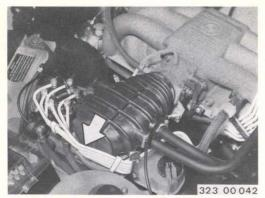
Check fuel lines at carburetors or fuel injection system for correct location, general condition and freedom from leaks.
