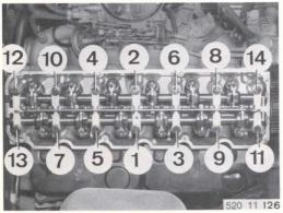
Max. engine temperature: +35°C (+95°F). Tighten cylinder head bolts one after the other in sequence 1... 14, in 2 stages: 1)
