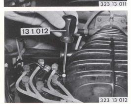
2) Adjusting CO level in % by volume Remove screw plugs from exhaust manifolds and insert test probes 13 0 020.
