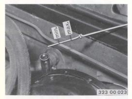
Automatic transmission – checking oil level
