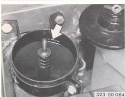
Checking power steering oil level: Stop engine. Remove wing nut and tank lid. Oil level must be app. 5 mm (0.2 in) above mark on inside of tank. Start engine. Add oil if necessary until level is
