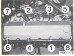
2. Tightening cylinder head bolts at 7500 km (5000 miles); this job is not part of any later Oil Service
