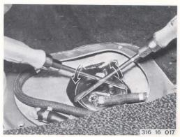
When installing: clean fuel strainer. The round cord seal swells when in contact with gasoline and in this manner provides a perfect seal. Check round cord seal and renew if necessary.
