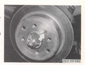
Check minimum thickness and condition of linings.
