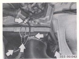
Fuel injection engine: Unscrew the pipe. Detach air inlet trumpet. Release snap fasteners.
