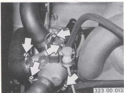
Tighten all hose clips on engine.
