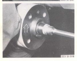
Tighten castle nut to 30...33 Nm (22...24 ft. lb) while constantly turning the wheel.
