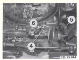
Checking function of stage II damper
