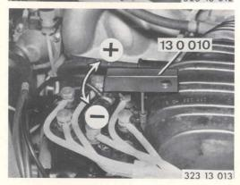
Adjust the CO value<sup>1</sup>) with adjusting wrench 13 0 010.
