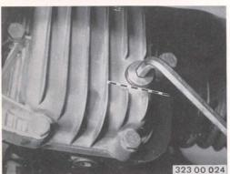
3. Checking/correcting final drive oil level Unscrew oil filler plug with 10 mm socket wrench.
