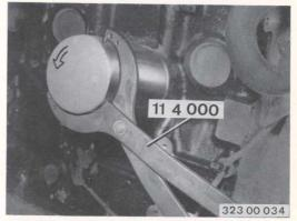
For version with air conditioning: Unscrew adaptor with 32 mm (1<sup>1</sup>/<sub>4</sub> in) wrench and separate filter from adaptor.
