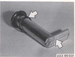
Carburetor engine: Clean strainer in fuel pump. Loosen screw (1).
