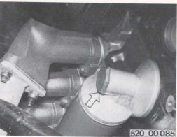
When installing: Insert adaptor in lock. Renew aluminum seal.
