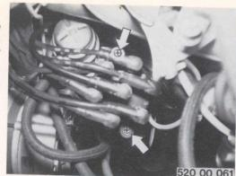
Remove the distributor rotor and dust cover.
