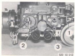
With mixture regulating screws (2 and 3), adjust the CO level in the exhaust 1).
