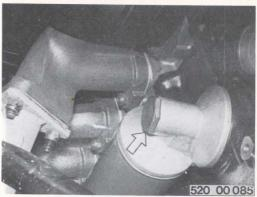
When installing: Place adaptor in lock. Renew aluminum seal. Tightening torque: 1)
